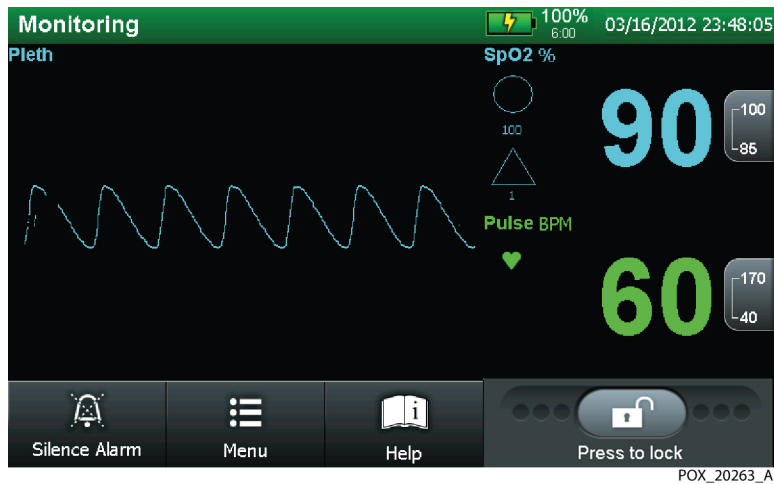
Figure 10-17. LIGHT Test: BPM 60, SpO2 90, MOD low, Light High
